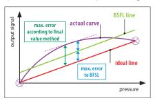
Non-linearity is also shown as BFSL (Best Fit Straight Line) as a reference value in the technical specifications. Non-linearity generally has the biggest influence on the overall error rate. Typically, non-linearity as per BFSL corresponds to half of non-linearity as per the full scale method (1% FS  $\sim$  0.5% BFSL).
